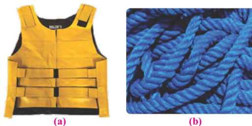
(a) (b) Figure 26.1 a) A bulletproof vest made from Kevlar ® b) poly(propene) rope
