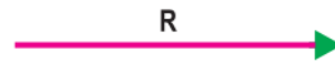
Fig.17.11(c): Vector diagram of RLC-series circuit showing that it behaves as pure resistive R-circuit at X_L = X_C
