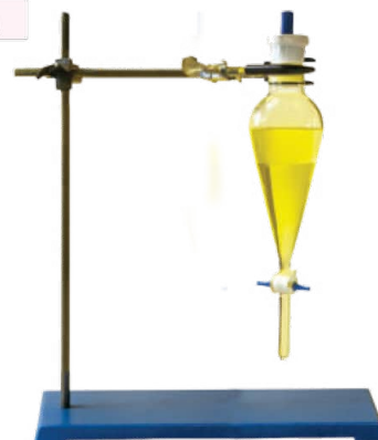
Fig. 15.1: Separating funnel used for the separation of immiscible liquids
