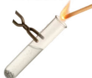
Fig.16.4: Hydrogen gas produces a faint 'pop' sound when ignited with a burning wooden splint
