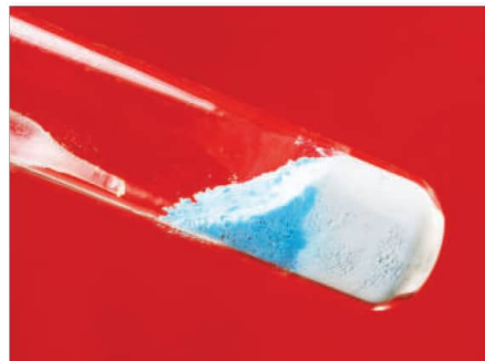
Fig. 11.8: Test for the presence of water
