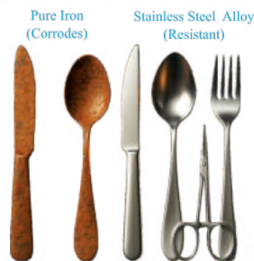
Fig. 6.4: Pure iron corrodes, whereas stainless steel alloy resists corrosion.
