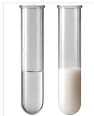
Fig.16.2: Carbon dioxide turns clear limewater milky because of the formation of calcium carbonate
