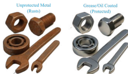
Fig. 6.5: Grease or oil coating protects metal from rusting.
