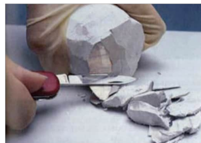
Fig. 10.6: Sodium is a soft metal and can be cut by a knife
