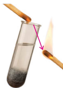
Fig.16.5: A glowing splint reignites when it contacts oxygen gas, confirming its presence.
