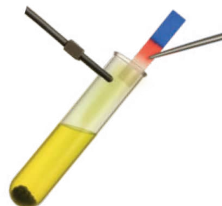
Fig.16.3: Chlorine gas causes damp blue litmus paper to turn red and then bleach it white.
