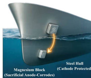
Fig. 6.9: Magnesium anodes corrode to protect the steel hull from rusting.
