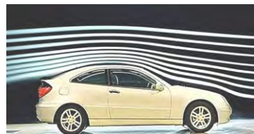
Fig. 3.11 Streamline air flow over a speedy car
